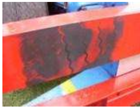
The rear bumper showing tyre marks
